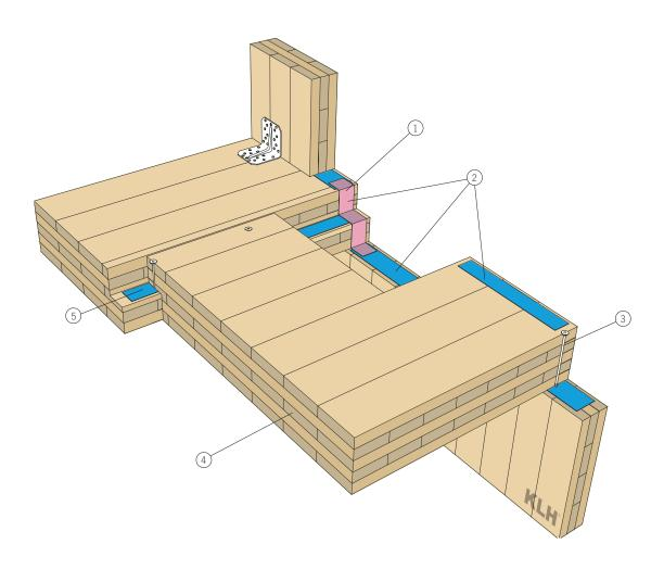
1 Arrange sealing strips laterally to the stepped profile
